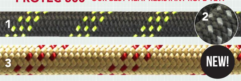
The ProTec 500 is a new CE EN1891 Type A certified 11mm semi static rope with a Technora® cover, essential for all Rope Access professionals who require a work positioning rope with outstanding heat resistant properties. The hi-visibility indicators will melt/fuse if exposed to temperatures over 250°c (482°F), providing visual and tactile evidence of high temperature exposure. Ideal for use around hot pipes and in welding operations.
